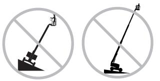
Do not depend on the tilt alarm as a level indicator. The tilt alarm sounds in the platform only when the machine is on a severe slope.
